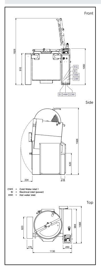
High Productivity Cooking Smart Electric Boiling Pan 150lt, 600mm tillting height
